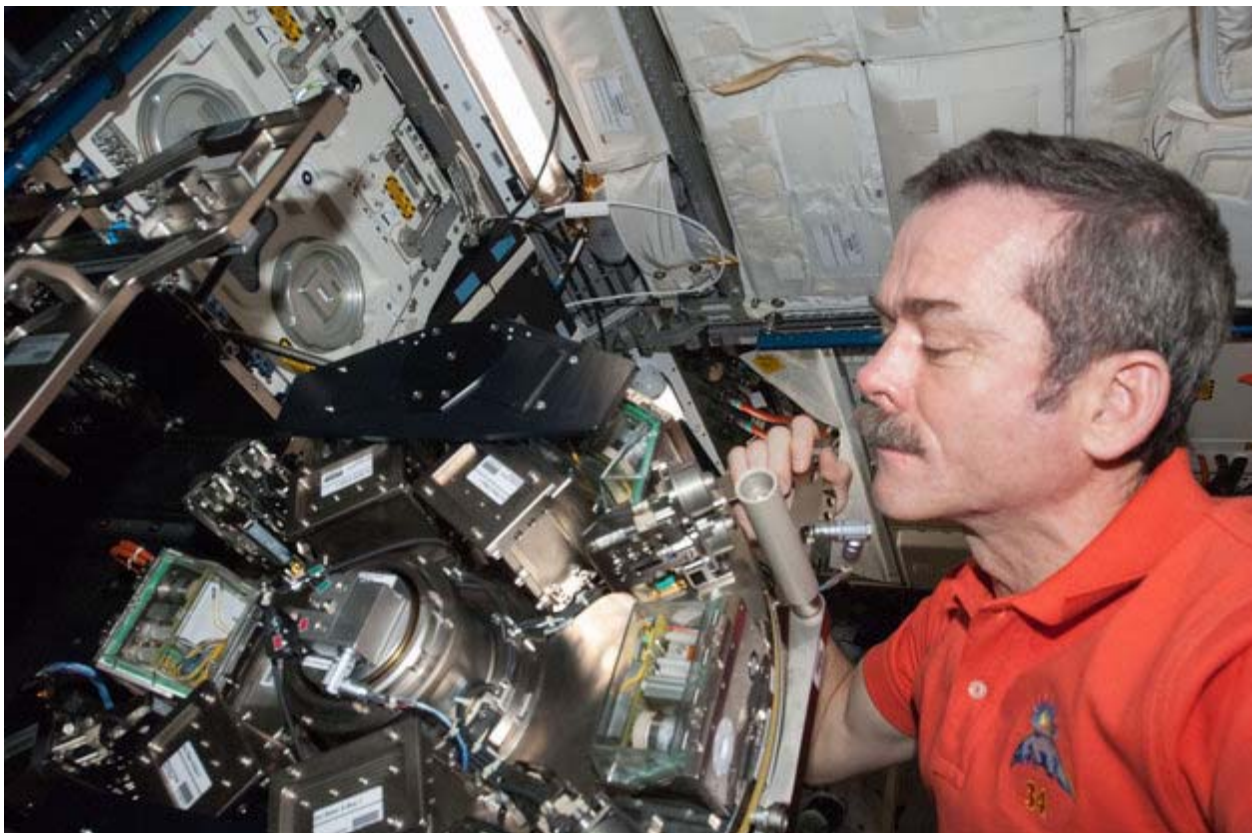
Figure: Astronaut Chris Hadfield inspecting one of the Biolab rotors. Individual IEC experiment containers (transparent) can be seen attached to the outer edge of the rotor.
