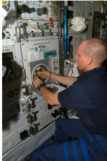
Figure: US Astronaut Clayton Anderson working with samples in the Refrigerated Centrifuge on board ISS.
