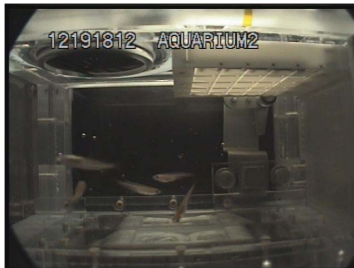
Figure: Medaka fish in the Aquatic Habitat in the Kibo Module are fed by the automatic feeder. Photo is the 55th day after the experiment starts in space.
