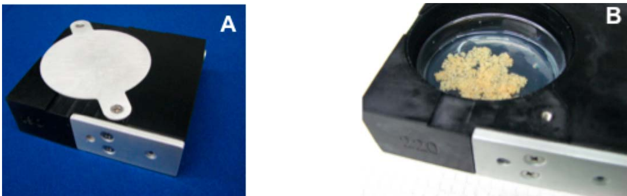
Figure: (A) View of an assembled Petri Dish Fixation Unit (PDFU). (B) Callus culture on petri dish within a PDFU prior to closure (see Paul et. al., 2012).
