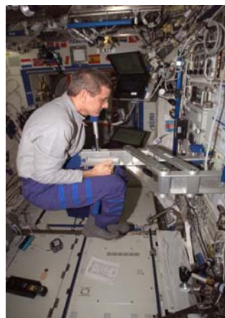
Figure: US Astronaut Bill McArthur performs a body mass measurement on board the ISS using the SLAMMD
